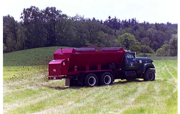
Ogunquit wastewater treatment facility operators use a specialized town truck to apply Ogunquit biosolids on nearby farm fields.
